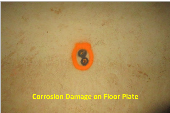
Corrosion Damage on Floor Patch Plate Weld and Floor Plate Weld Joint
